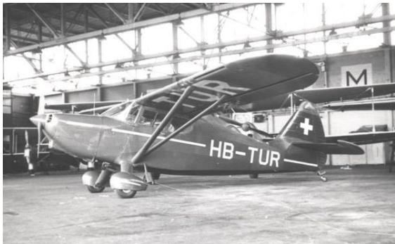
Swiss Stinson 108-2 at Manchester Airport, England in 1950. This earlier model has the shorter vertical fin with curved trailing edge.
