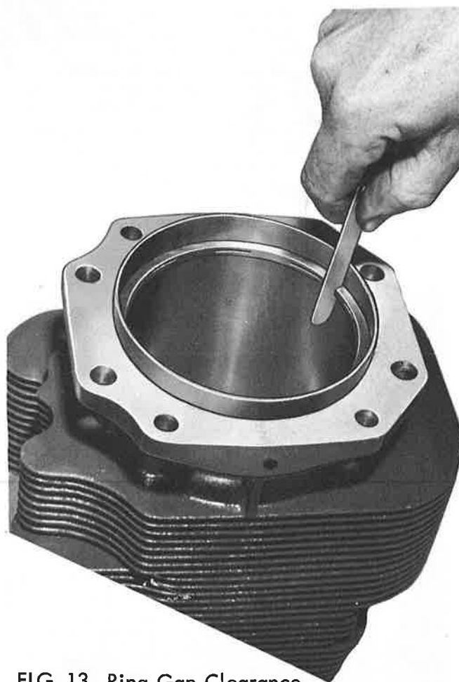
FIG. 13. Ring Gap Clearance
