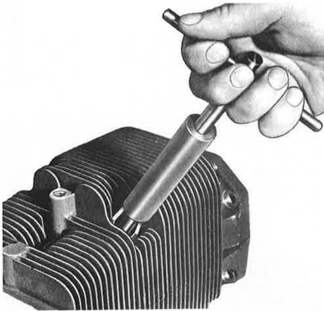
3. Installing the Helicoil Insert
