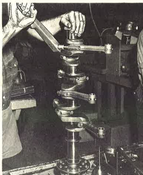
FIG. 47. Torquing Connecting Rod Bolt
